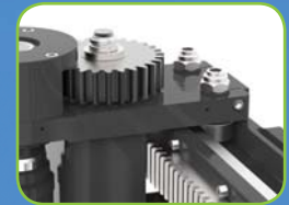
Eccentric roller pins adjust tolerance between rack & pinion to maintain smoothness
